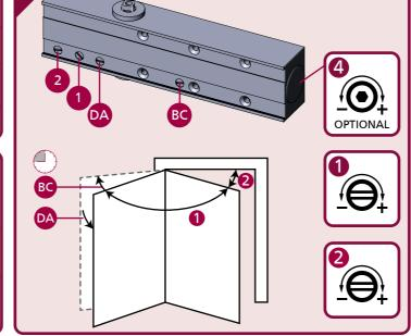
DELAYED ACTION & BACK CHECK (DABC) VALVES ARE NOT STANDARD, THESE ARE OPTIONAL. FOR UNINSULATED STEEL DOORS IP.95M MUST BE USED. THE PINION BOLT MUST BE TIGHTENED TO 12Nm.
