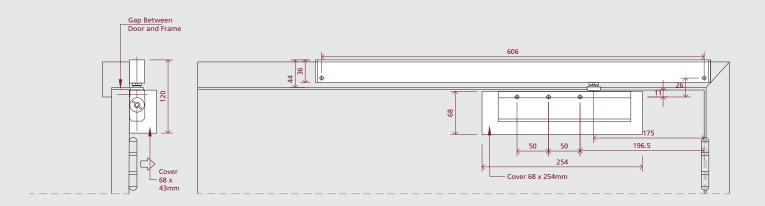
When E-mag door closers are to be interfaced with fire & smoke alarm systems they are to be installed by competent installers in accord with BS 7273-4 code of practice.
