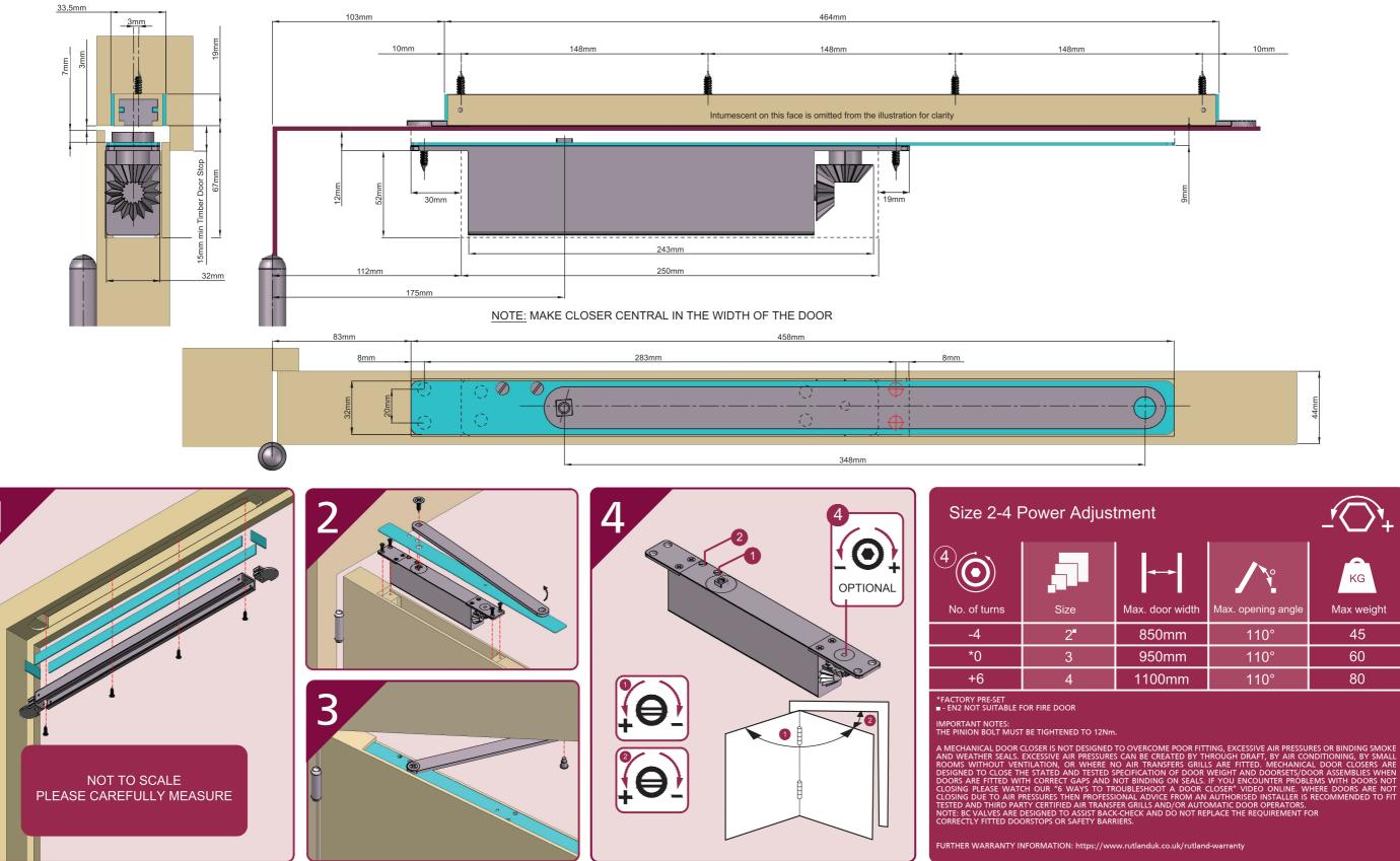
THE PINION BOLT MUST BE TIGHTENED TO 12NM FIRE DOORS MUST BE FITTED WITH INTUMESCENT GASKETS
